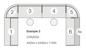
1: CONR16/AE Rectangular Workstation with Accessibility Extension 2: CONCN/INTLH Corner Workstation with Inset Leg 3: CONR14/INT Rectangular Workstation with Inset Leg 4: CONR14/INT Rectangular Workstation with Double Inset Legs 5: CONCN/INT Corner Workstation with Double Inset Legs 6: CONR16/INTRH Rectangular Workstation with Inset Leg CON/CTR16/38 6a: Rectangular Counter Top
