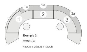
1: CONCV/AELH Curved Workstation with Accessibility Extension 1a: CON/CTCV/T38 Curved Third Counter Top 2: CONR12 Rectangular Workstation 2a: CON/CTR12/38 Rectangular Counter Top 3: CONCV/AERH Curved Workstation with Accessibility Extension
