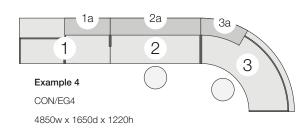
CONR16/ASLH Rectangular Workstation with Inset Leg and Accessibility Section CON/CTR8/48 1a: Rectangular Counter Top CONR16/INTRH Rectangular Workstation with Inset Leg
