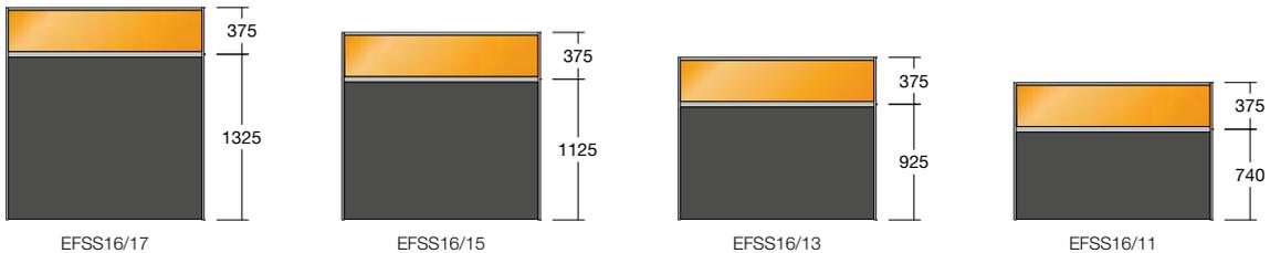
The above illustrations show the fabric / MFC and acrylic portions of the Elite half glazed floor standing system screen as standard.
