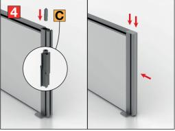
**4.** Secure the top link (C) ensuring that the screen or link post are aligned.
