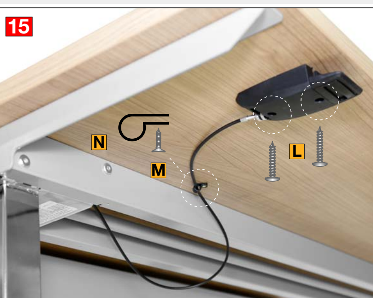
15. Attach the release lever to the underside of the top with 2 x 'L' Screws, pilot holes are pre-drilled for guidance. Fix the cable to the underside of the top as illustrated with the cable clip provided, see items 'N' & 'M'.
