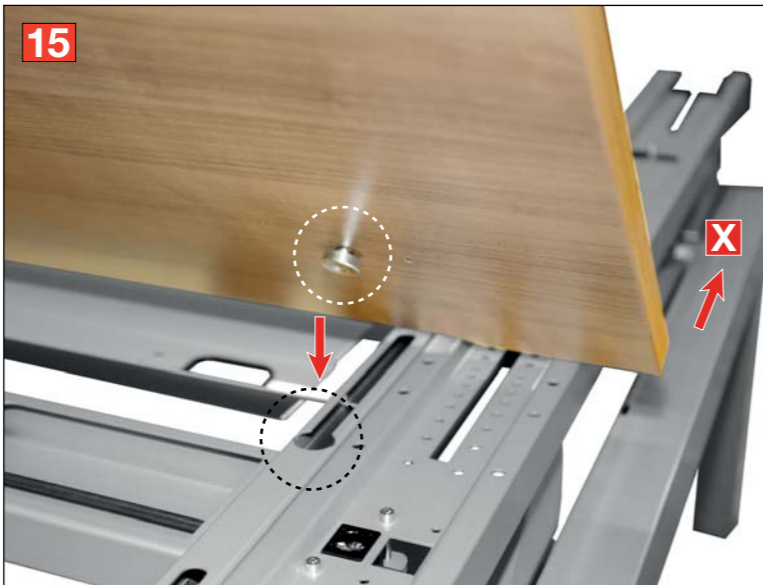
15. Place each Top Panel (A) above the keyhole slots in the Underframe (C). Slowly lower into place. Once located, slide the top in the direction of arrow X.
